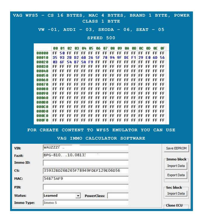
ADAPTATION: FOR PROPER OPERATION OF THE EMULATOR SAVE THE IMMOBILIZER DATA IN ITS MEMORY (24C02 ON PCB), TWO DATA SETS SUITABLE FOR ECU AND TCU, IN THE CASE OF USING THE EMULATOR TO DISARM BOTH DRIVERS AT THE SAME TIME.
